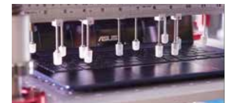
Keyboard Test To ensure ultimate keyboard durability, specially designed ASUS robots test individual keys with millions of keystrokes.
