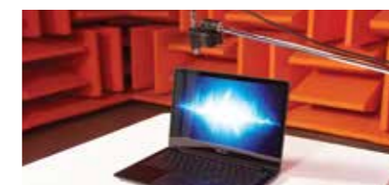
Noise and Audio Test Laptops undergo fan, hard drive, and power-supply noise tests to ensure the quietest performance possible.
