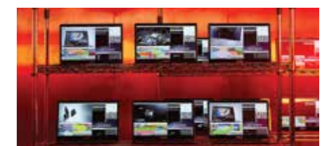
Temperature Test Extremely high or low temperatures tests ensure laptop functions consistently for users everywhere.
