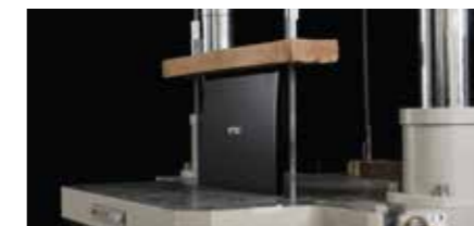
Shock Test Shock tests ensure a laptop can withstand unexpected impacts such as accidental bumps, or jarring movements during shipping.
